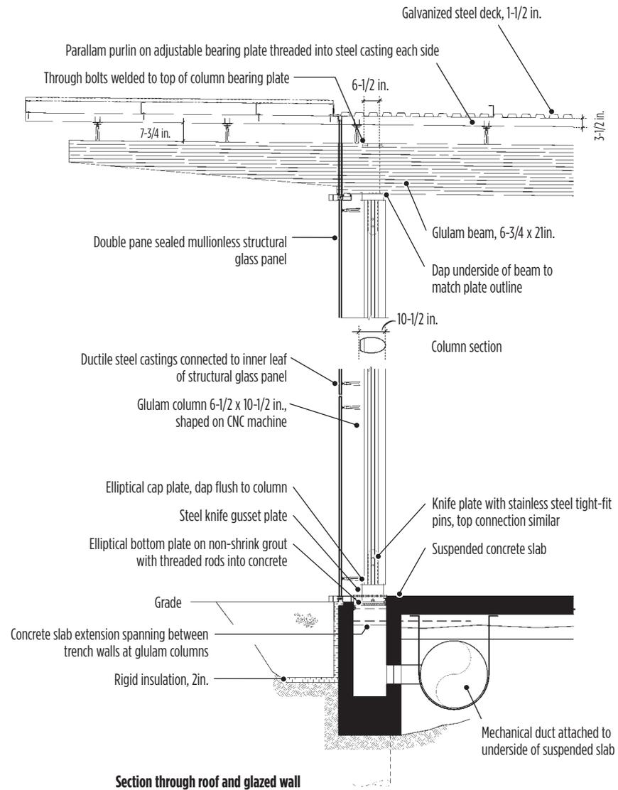
**Section through roof and glazed wall**
