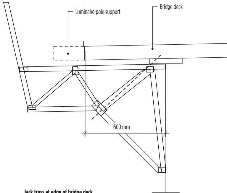
**Jack truss at edge of bridge deck**
