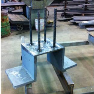
The column-to-column connector with saddles to carry glulam beams *Courtesy: Fast + Epp*
