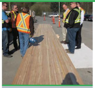
Factory prefabrication of nail-laminated floor panels Courtesy: Proscenium Architecture
