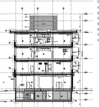
CLT Enclosure Band Option - Section at loading bay looking east Courtesy: Fast + Epp
