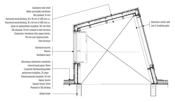
Section through research wing roof monitor
